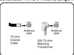
Connect the 75 ohm cable from the combination VHF/
